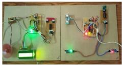
Here, the ERV and non-ERV are displayed in working state where ERV acts as a sender and non-ERV acts as a receiver. In order to replicate the speed of a vehicle, we use a DC motor. The ultrasonic sensor used in this project detects the automatic distance of the nearby vehicle and sends the information to the non-ERV which is displayed on the LCD display.
